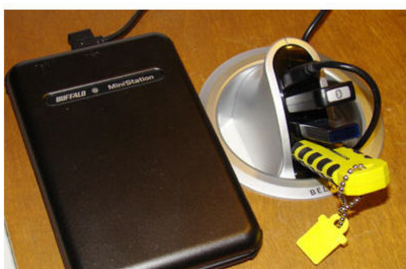
Belkin In-Desk USB hub installed and fully loaded.
